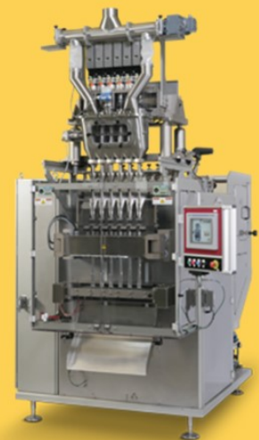
VERTICAL FORM FILL SEAL
